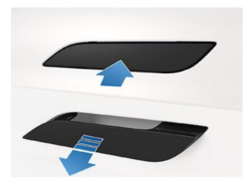
Insert your hand into the handle and pull to open the door.
