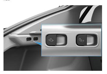
To return the seats to their upright position, pull upwards until it locks into place. To confirm that the seat is locked in the upright position, try pulling it forward.
