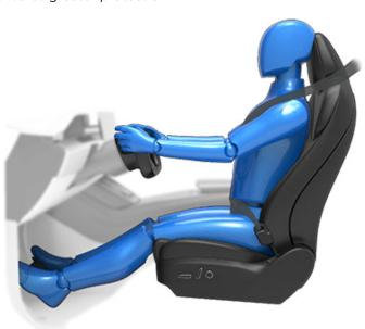
Position the seat so you can wear the seat belt correctly, while being as far away from the front airbag as possible:
