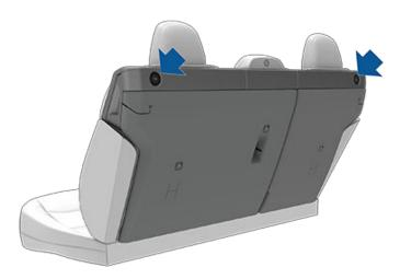
You can also fold the rear seats fully forward by pressing the corresponding switch located on the left side of the rear trunk. Pressing the switch causes the seat to unlatch. You can then push it downward to lay it fully
