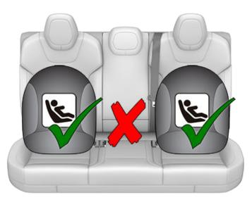
To install a LATCH child safety seat, lift the flap (if equipped) to allow access to the anchors.
