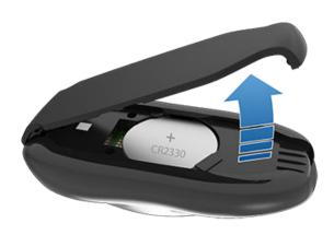
2. Remove the battery by lifting it away from the retaining clips.
