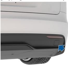
3. Fully insert the tow eye into the opening, then turn it **counter-clockwise** until securely fastened.
