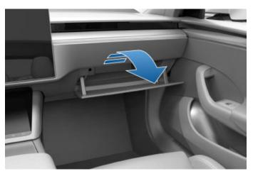
To close the glovebox, push it upward until it latches into the closed position.
