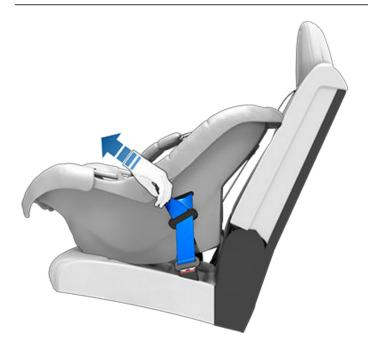
Before seating a child, ensure that the child restraint system is securely installed. Grasp the front of the child restraint system with one hand on each side, and attempt to:
