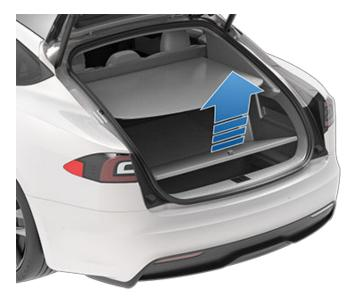
The cargo weight should be distributed as evenly as possible between the front and rear trunks.
