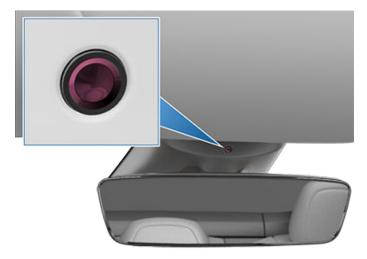
**NOTE:** Keep the camera lens clean and free of obstructions. Remove any buildup of dirt or dust by occasionally wiping the camera lens with a clean cloth.
