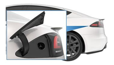
**NOTE:** The charge port lights up white when you open the charge port door. If you do not insert a charge cable into the charge port within a few minutes after opening the charge port door, the charge port door closes. If this happens, use the touchscreen to open the charge port door again.
