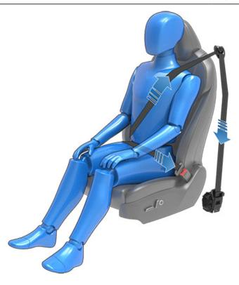
If the pre-tensioners and airbags did not activate in an impact, this does not mean they malfunctioned. It usually means that the strength or type of force needed to activate them was not present.
