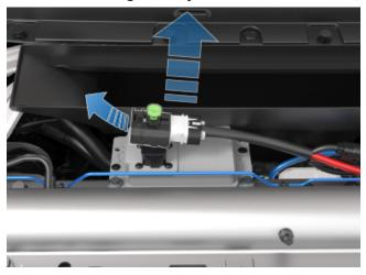
5. Release the cover from the red positive (+) jump post, and then connect the low voltage power supply's red positive (+) cable to the red positive (+) jump post.
