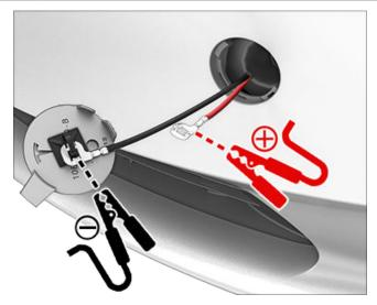
**NOTE:** Applying external low voltage power to these terminals only releases the hood latches. You cannot charge the low voltage battery using these terminals.
