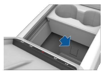
The power socket is suitable for accessories requiring up to 12A continuous draw (16A peak).
