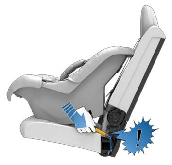
Adjust until the child restraint system is fitted firmly against the seat back. Ensure the child restraint system fits snugly.
