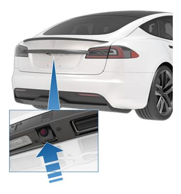
Whenever you shift into Reverse, the touchscreen displays the view from the camera. Lines show your driving path based on the position of the steering yoke (or steering wheel). These lines adjust as you move the steering yoke (or steering wheel).
