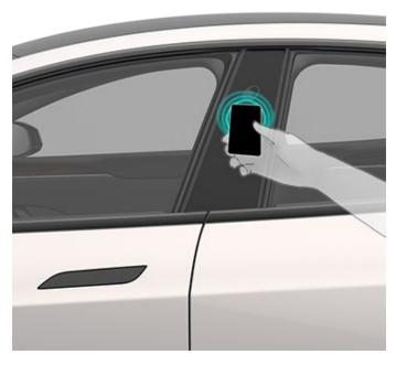
Once inside, power up Model S by pressing the brake pedal within two minutes of scanning the key card (see Starting and Powering Off on page 53). If you wait longer than two minutes, you must re-authenticate by placing the key card near the card reader located in the wireless phone charger on the center console. When your key card is detected, your two minute authentication period restarts.
