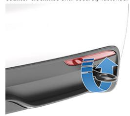
4. Attach the winch cable to the tow eye.
