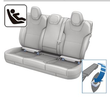
In the rear seats, install LATCH child safety seats in the outboard seating positions only. Use only a seat belt retained seat in the center position.
