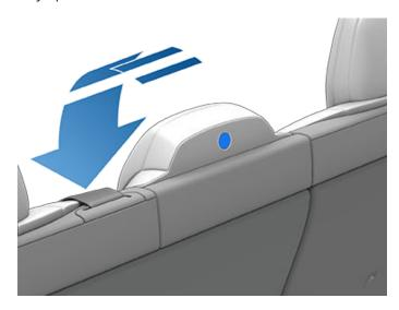
To access the storage tray and wireless phone charger (see Wireless Phone Chargers on page 26), raise the cover by pressing the latch on the underside of it and pulling it up.
