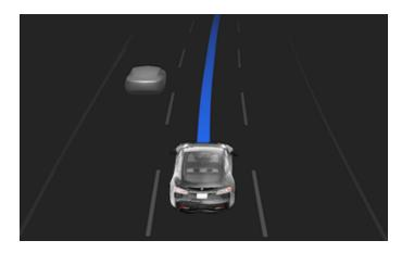
When Navigate on Autopilot is active and you approach an off-ramp or interchange along your navigation route, the appropriate turn signal engages and Autosteer maneuvers Model S onto the off-ramp or interchange.
