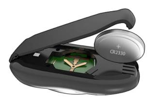
3. While avoiding touching the battery's flat surfaces, insert the new battery (type CR2330) with the '+' side facing up.
