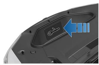
2. Release the front tow eye cover by pressing firmly on its top right perimeter until it pivots inward, then gently pulling the raised section toward you.
