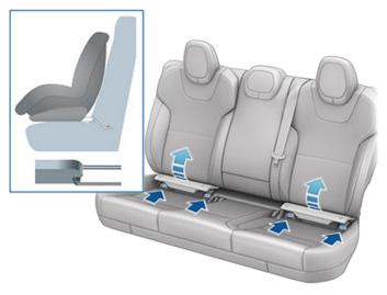
Carefully read and follow the instructions provided by the manufacturer of the child restraint system. The instructions describe how to slide the child restraint system onto the seat's anchor bars until you hear it "click" into place. You may need to push the child restraint system firmly against the seat back to ensure it fits snugly. The flap (if equipped) remains open when the child seat is installed.
