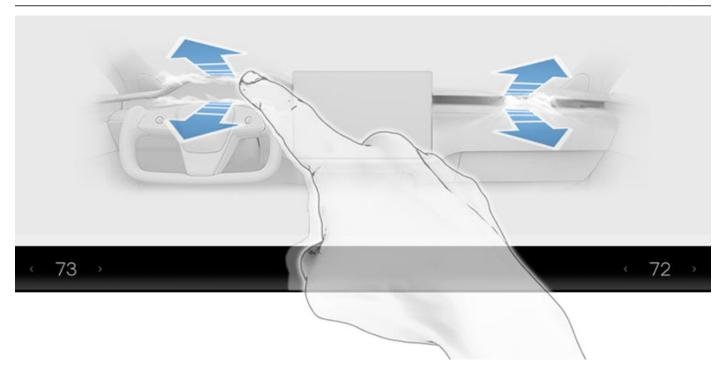
**NOTE:** When you split a vent into two separate air flows, the air flow in each direction is not as strong as when all air is flowing in a single direction.
