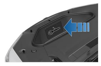
Release the rear tow eye cover by pressing firmly on its bottom perimeter until it pivots inward, then gently pulling the raised section toward you.
