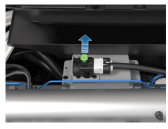
4. On top of the low voltage battery, pull the connector housing to the left. The electrical connector releases from the low voltage battery.
