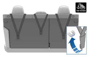
Position single-strap tethers for the outboard seating positions to run on the outside of the head support. Position a single strap in the center seating position to run over the top of the seat as illustrated.
