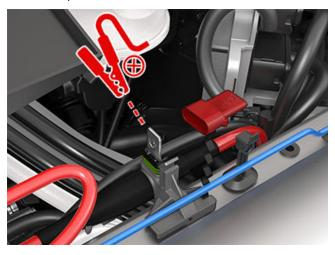
Connect the low voltage power supply's black negative (-) cable to the vehicle in the location shown.
