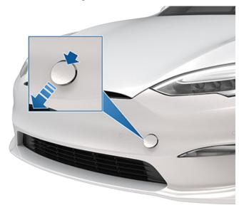
3. Fully insert the tow eye into the opening, then turn it **counter-clockwise** until securely fastened.
