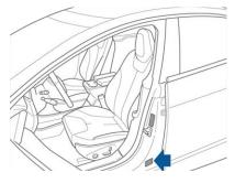
Stamped on the chassis under the sill panel on the rear passenger door. To remove the sill panel, gently pry it upward using a flat-bladed tool.
