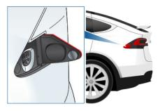
**Note:** The charge port lights up white when you open the charge port door. If you do not insert a charge cable into the charge port within a few minutes after opening the charge port door, the charge port door closes. If this happens, use the touchscreen to open the charge port door again.
