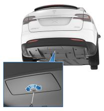
Note: Newer versions of Model X have two push clips that secure the dust cover to the vehicle. To open, use a sharp object, such as a flat screwdriver, to carefully pry the clips open. Remove the dust cover.
