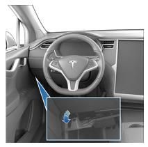
**3.** Peel back the carpet to expose Model X's 4-pin connector on the wiring harness.
