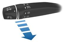
Autosteer briefly displays a message on the instrument panel reminding you to pay attention to the road and be ready to take over at any time. To indicate that Autosteer is now actively steering Model X, the instrument panel displays the Autosteer icon in blue. When Autosteer is able to detect lane markings, it also displays the driving lane in blue.
