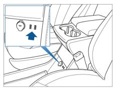
In addition, Model X has two charge-only USB ports located at the rear of the center console, and another charge-only connection located between the third row seats.
