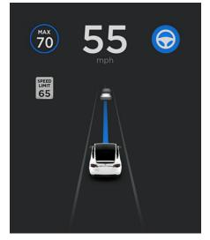
When Navigate on Autopilot is active and you approach an off-ramp or freeway interchange along your navigation route, the appropriate turn signal engages and Autosteer maneuvers Model X onto the off-ramp or interchange.
