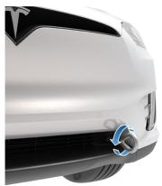
4. Attach the winch cable to the tow eye.
