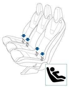
In the second row, install LATCH child safety seats in the outboard seating positions only. Use only a seat belt retained seat in the center position.
