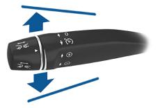
To set the cruising speed to the speed limit plus any offset you've specified using Speed Assist, pull the cruise control lever toward you. If you are already driving faster than the speed limit, the set speed does not adjust to the speed limit—it adjusts to your current driving speed. If you move the cruise control level up or down after setting Traffic-Aware Cruise Control to cruise at the speed limit, your set speed becomes your current driving speed.
