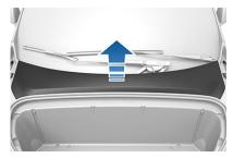
Caution: The maintenance panel protects the front trunk from water. When reattaching, make sure it is fully seated.
