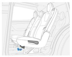
**Note:** You can adjust the position of bench seats using the mechanical levers only. You cannot use the touchscreen to adjust bench seats.
