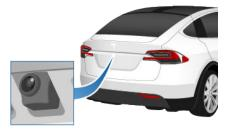
Whenever you shift into Reverse, the touchscreen displays the view from the camera. Lines show your driving path based on the position of the steering wheel. These lines adjust appropriately as you move the steering wheel.
