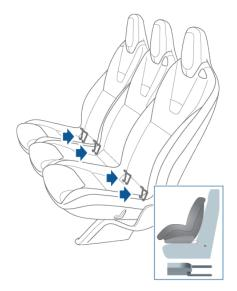
Once installed, test the security of the installation before seating a child. Attempt to twist the child safety seat from side to side and try to pull it away from the seat, then check to ensure the anchors remain securely in place.
