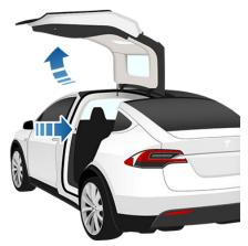
**Note:** If Model X is locked, using the switch (illustrated above) the first time unlocks the associated door. Pulling it a second time opens it.
