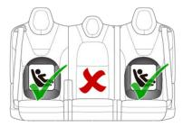
**Note:** To accommodate large rear-facing LATCH child safety seats, you may need to move the seat in the full rearward position, and move the corresponding front seat forward to the mid-track position (up to 13 cm forward of the rearmost position), raise the seat upward (3 cm from its lowest position), and angle the seat back to 15 degrees (or 10 degrees rearward from its forward-most position).
