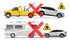
Do not transport Model X using any method that is not specified by Tesla. Adhere to the instructions provided in the following sections and observe all warnings and cautions provided. Damage caused by improper transporting of your vehicle is not covered by the warranty.
