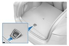
Caution: Never load more than 175 lbs (80 kg) on the rear load floor (above the lower trunk compartment) or more than
