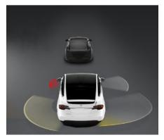
Lane Assist also warns you when a desired lane departure is not appropriate. When you engage the turn signal and a vehicle or object is detected in the adjacent lane you are planning to move into, the instrument panel displays a red lane line to indicate that a vehicle or object is detected. When the vehicle or object is no longer detected, the lane line returns to normal.
