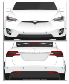
The sensors are activated when driving slower than 5 mph (8 km/h).
