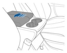
To expose rear cup holders (if available on your vehicle), press and release the cup holder face plate located at the back of the center console.
