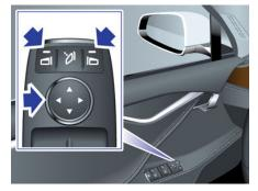
To fold and unfold exterior mirrors, press the center button. You can set the mirrors to fold automatically whenever Model X is locked by touching **Controls > Vehicle > Mirror Auto-Fold**. The mirrors unfold automatically whenever you unlock Model X.
