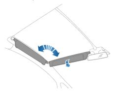
To expose the vanity mirror, lower the visor extender then lower the mirror cover. While the cover is lowered, the mirror is exposed and lights are illuminated.
