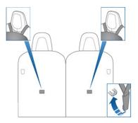
For single-strap tethers, position the strap in the outboard seating positions over the outside-facing side of the head restraint (the same side of the head restraint as the seat belt retraction mechanism). In the center seating position (if equipped), center and position the strap over the top of the head restraint.
