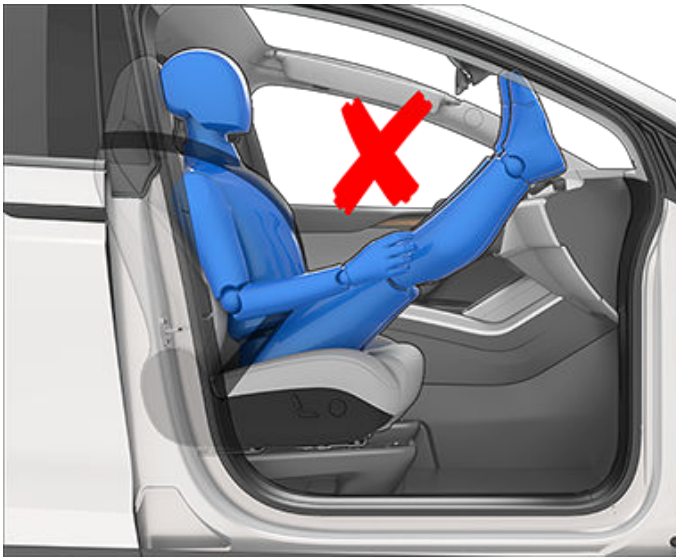
Incorrect seating position - the passenger must not slide forward on the seat cushion:
